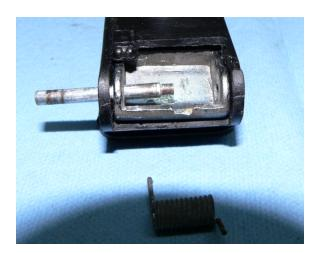
14. Lay the spring into the end of the latch-lever while slipping the end of the spring over the small end of the hinge pin. Make sure the spring arm with the bent end fits between the two round bosses protruding from the housing's bottom edge.
